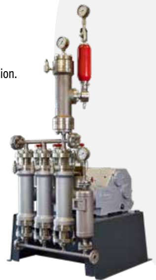
FELUWA MULTISAFE® double hose-diaphragm pump Example application: TG 135 – 3 DS 100 Triplex, single-acting pump: 24 to 47 m³/h at 70 bar and 100 °C Medium: aggressive and abrasive chemical catalyst Media-contacting components made of 1.4410 (Super Duplex) and hose-diaphragms of EPDM
